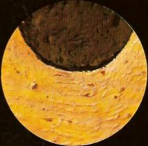
Rolled screw thread. Deformed structure. Brightfield on the left, differential interference contrast on the right. Metal
